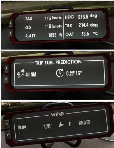
Precision navigation page. Note that the radar altimeter only works below 2000 ft AGL and with the wings roughly leveled.
