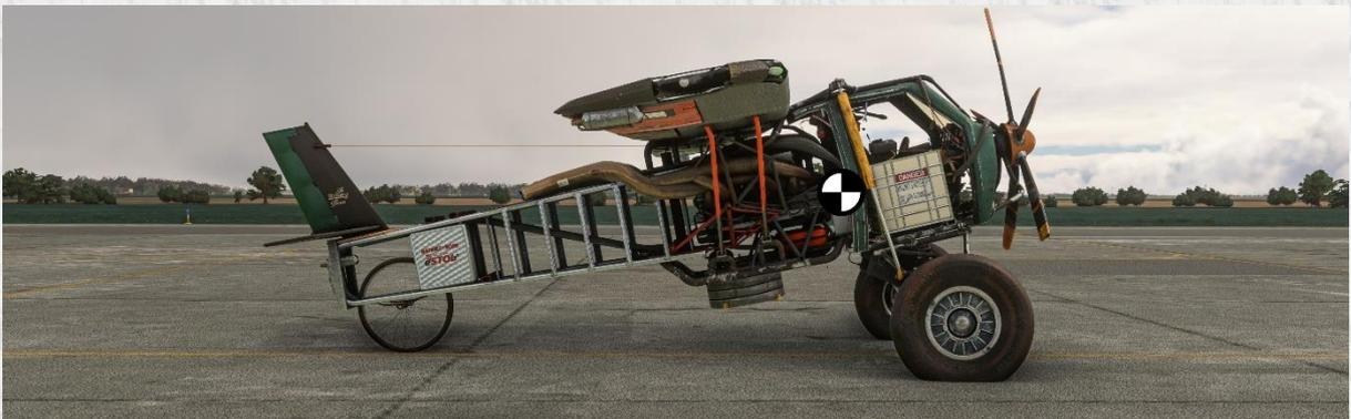
Also: The wings are relatively lightweight (fuel tank is located where the passenger seat would be in a normal aircraft). The weight is then not only centered on the roll axis, but also on the pitch axis. With all that, you end up with a **plane capable of doing aerobatics quite easily**.
