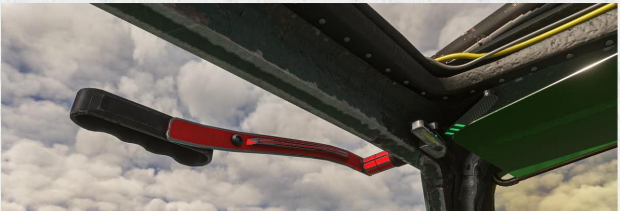
*On this picture, you have the flaps retracted (red lever up) and the automatic flaps retractor is already armed.*
